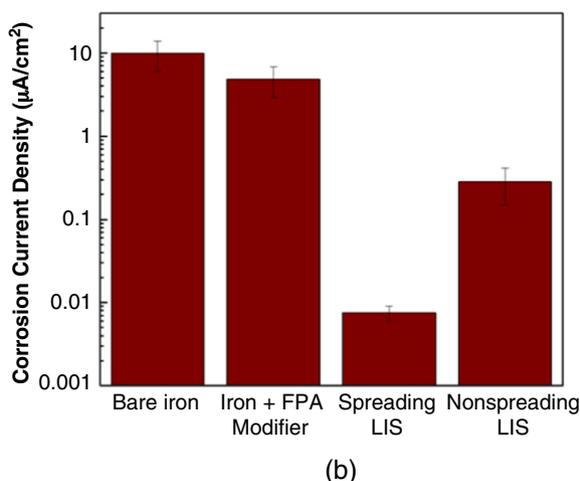
**FIGURE 4.** (a) Potentiodynamic polarization curves showing the open-circuit potential and (b) corrosion current density as determined from the potentiodynamic curves.
