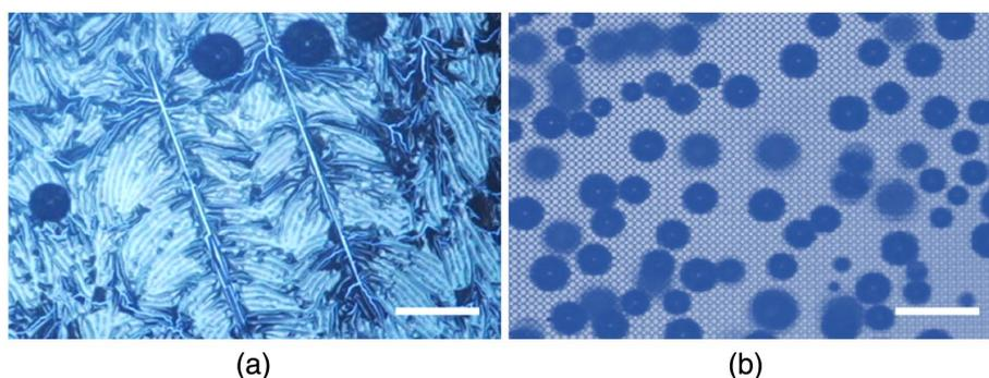
**FIGURE 2.** (a) A thin film of iron ( $0.5 \mu\text{m}$ ) on a smooth silicon wafer deteriorating when exposed to 0.1 M HCl, evolving hydrogen gas bubbles. (b) Iron film of the same thickness conformally deposited on textured silicon as shown in Figure 1(b), demonstrating even more vigorous bubbling when exposed to 0.1 M HCl. Scale bars are  $100 \mu\text{m}$ .
