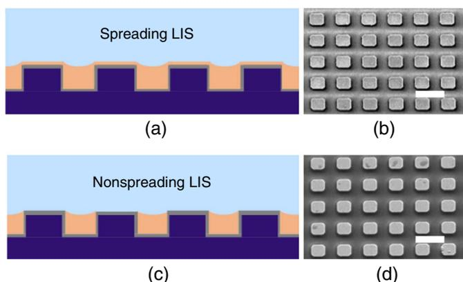
**FIGURE 3.** (a) Schematic showing a spreading LIS which covers both the tops and within the textures. (b) SEM image showing consistent lubricant coverage using the commercial lubricant which forms a spreading LIS. (c) Schematic showing a nonspreading LIS where the texture tops are exposed. (d) SEM image showing the nonspreading LIS made using silicone oil, showing discrete lubricant drops on top of posts. Scale bars shown are 20  $\mu\text{m}$ .
