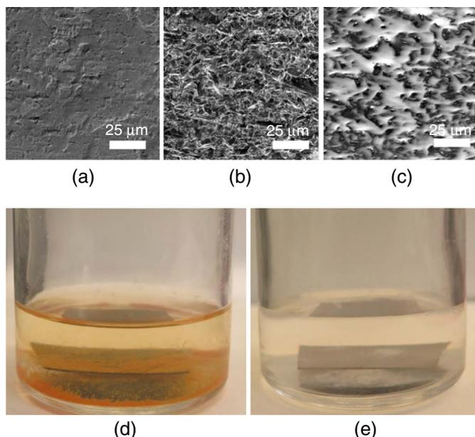
**FIGURE 5.** SEM images showing: (a) as-received carbon steel coupon, (b) sand-blasted coupon with micrometric roughness features, (c) the commercial lubricant-based spreading LIS developed on the textured coupon, (d) control coupon corroding after 48 h of exposure to 3.5 wt% NaCl, and (e) LIS-coated coupon showing no corrosion after 48 h.
