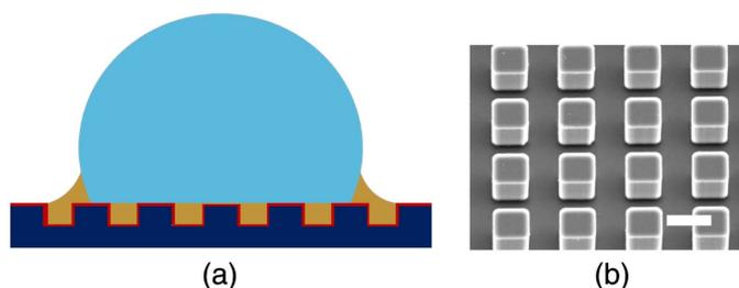
**FIGURE 1.** (a) Schematic of LIS showing a drop of water sitting atop a textured surface (dark blue) coated with a hydrophobic modifier (red layer) and impregnated with a lubricant (yellow). (b) Scanning electron microscopy (SEM) image of a microtextured surface on silicon showing pillars with width  $a = 10 \mu\text{m}$ , height  $h = 10 \mu\text{m}$ , and pitch  $b = 10 \mu\text{m}$ . Scale bar:  $15 \mu\text{m}$ .
